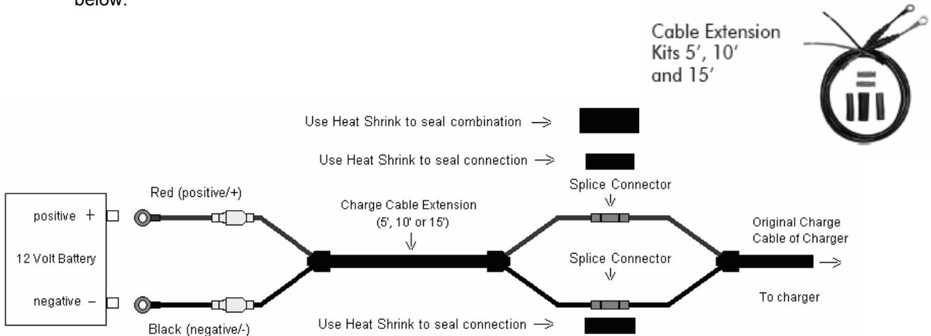
To connect the charger to the battery (batteries), route your charge cables from the charger to the batteries, being cautious to avoid sharp objects, and use the supplied wire ties to hold them securely and neatly in place.
