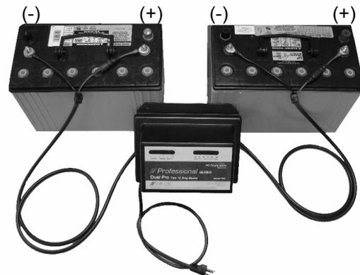
Connect a heavy duty UL approved extension cord to the power cord of your charger and then plug the extension cord into a nearby 120VAC GFI protected (Ground Fault Circuit Interrupt) outlet. You should now observe a red LED indication on each bank of the charger representing each individual battery being charged. The voltage of each battery will reflect the number of LED indicators illuminated.
